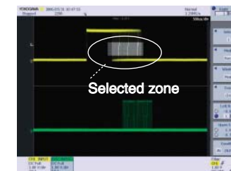
Zone search Define 1 to 4 zones and search for waveforms that fall inside or outside the zone (s).
